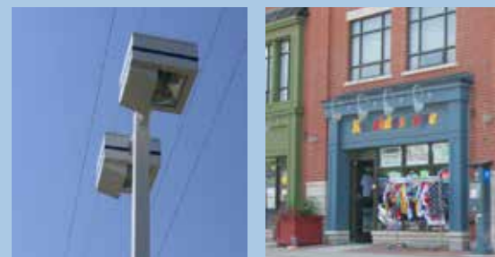
Examples of preferred lighting: (Left) shielded light fixture that cuts down on light trespass; (Right) lighting fixture above sign directed down.
